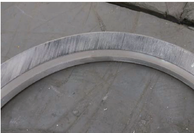
Damage to metal sealing system by metal sticking and creep deformation
