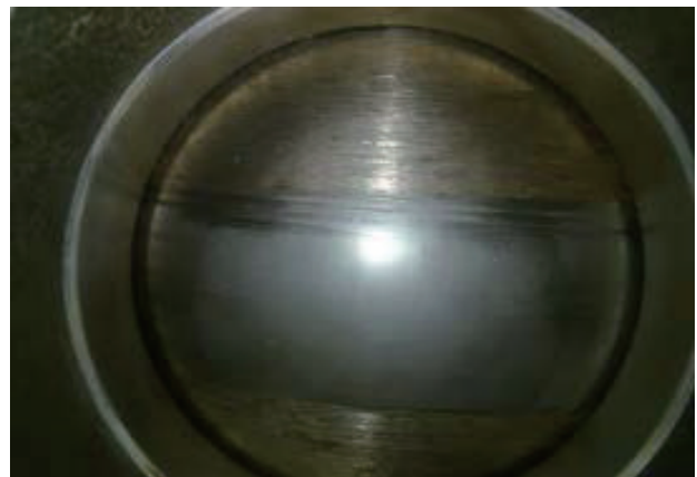
Damage to metal sealing system by metal sticking and creep deformation
