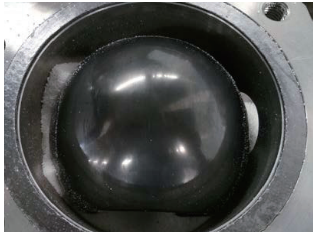
Fslloy30 sealing surface after 2 million cycles with polypropylene powder
