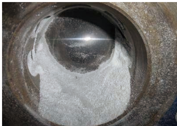
Fslloy28 coating surface after 800k cycles at polypropylene powder medium
