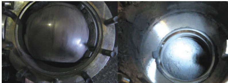
Valve ball and seat with F51+FSLLOY12 coating after 100000 times of opening/closings with dry coal powder medium
