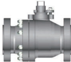
Model F2: Floating ball valve, 2-part cast valve body, full diameter structure design. The sealing of the middle flange is realized through the quantitative compression of the reliable sealing ring.
