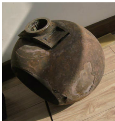
Damage of adhesion, corrosion and flushing to the hard sealing system
